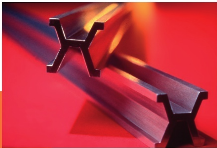
fig B A standard metre, made to be exactly the length that light could travel in 1/299\,792\,458 of a second.
