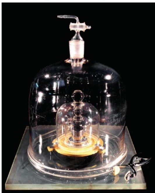
fig A The international standard kilogram, officially known as the International Prototype Kilogram, is made from a mixture of platinum and iridium and is held at the Bureau International des Poids et Mesures in Paris. All other masses are defined by comparing with this metal cylinder.
